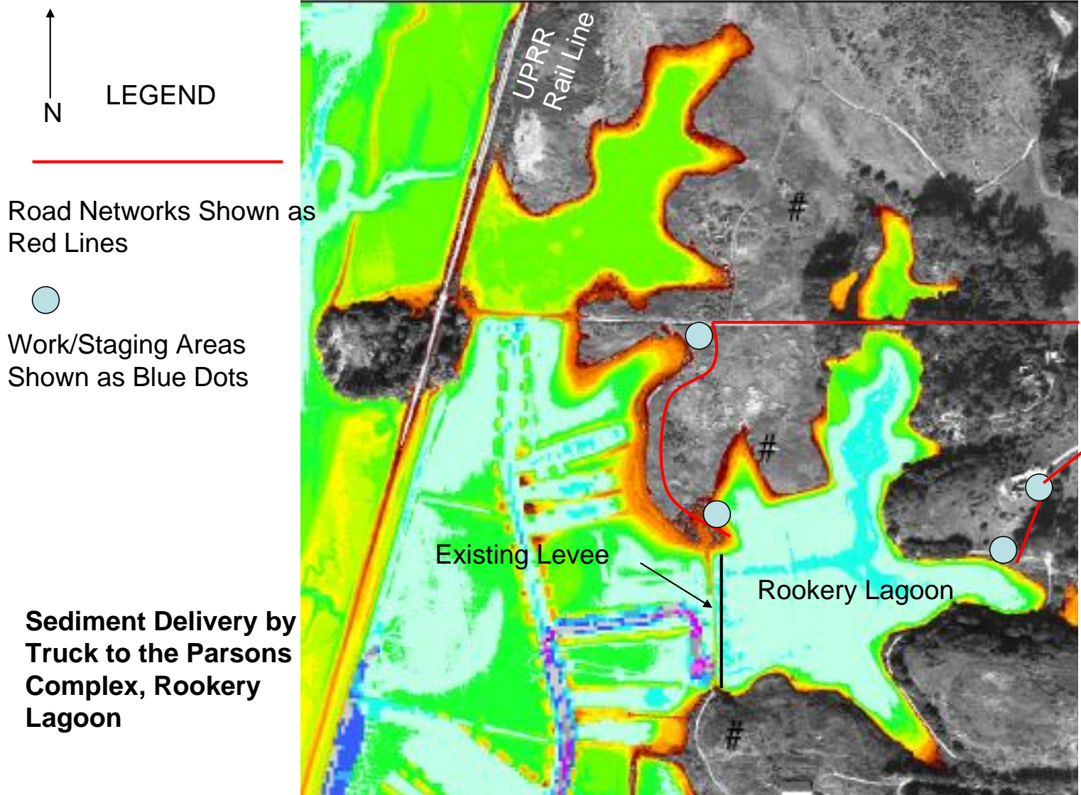
Figure 11 - Sediment Delivery by Truck and/or Scraper to Parsons Complex, Rookery Lagoon
